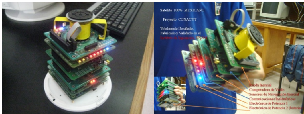
Figure 1. Developed Mexican PDS showing its architecture based in subsystem modularity.
